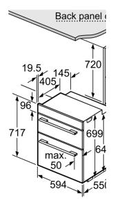
measurements in mm If the appliance will be a hob, the following w (including substructure be taken into account
