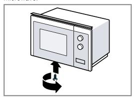
**4.** Loosen the two outer screws on the microwave base.
