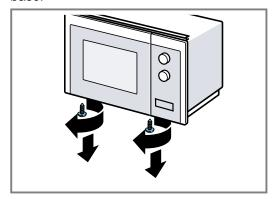
5. Secure the built-in frame on the microwave base with the two outer screws.
