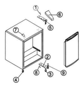
Remove the upper hinge cover (6) screws (1) and hinge (5) Lift the door away from the lower hinge
