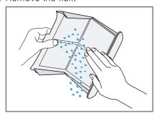
7. Clean the fluff filter thoroughly under warm, running water and then dry it off.
