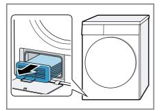
Clean the heat exchanger from all sides under running water and dry it.
