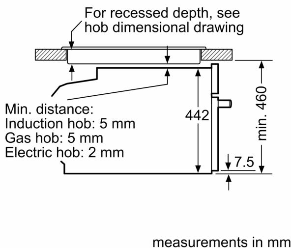
If the compact appliance will be installed underneath a hob, the following worktop thicknesses (including substructure if necessary) must be taken into account.
